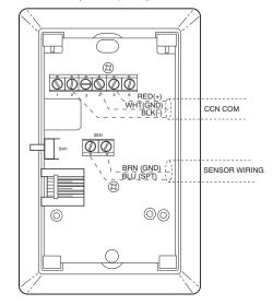
Fig. 43 - T-55 Space Temperature Sensor Wiring
